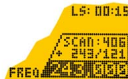
Scanning mode, switched to second scan-frequency (active frequency 243,000 MHz)
