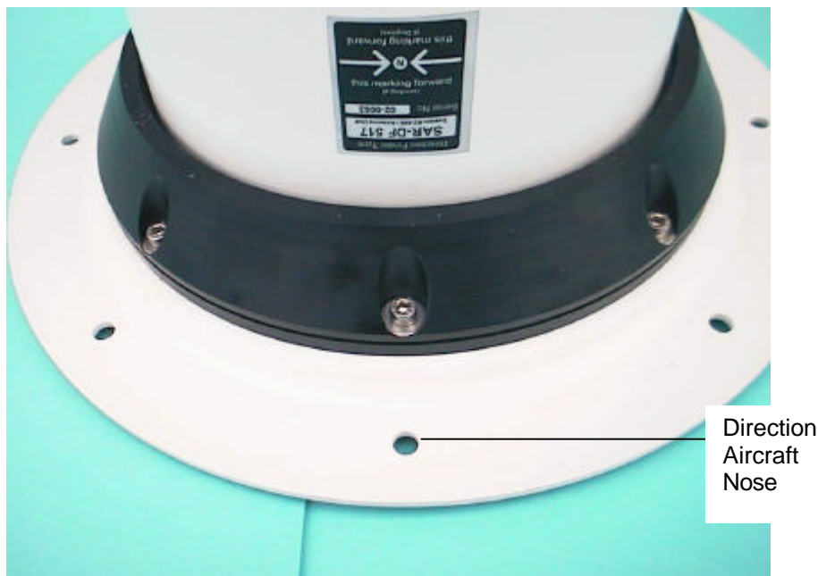
Fig. 2-5 Montage direction of the antenna unit
